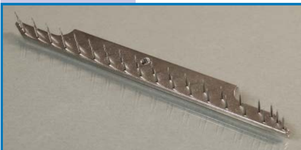
Dim 118 x 12 x 3.5mm 36 V3M pins Nr 20 x 11mm 80° setting 1 x M4 + 2 x 4mm buttons on the backside Part number 753.4013.361
